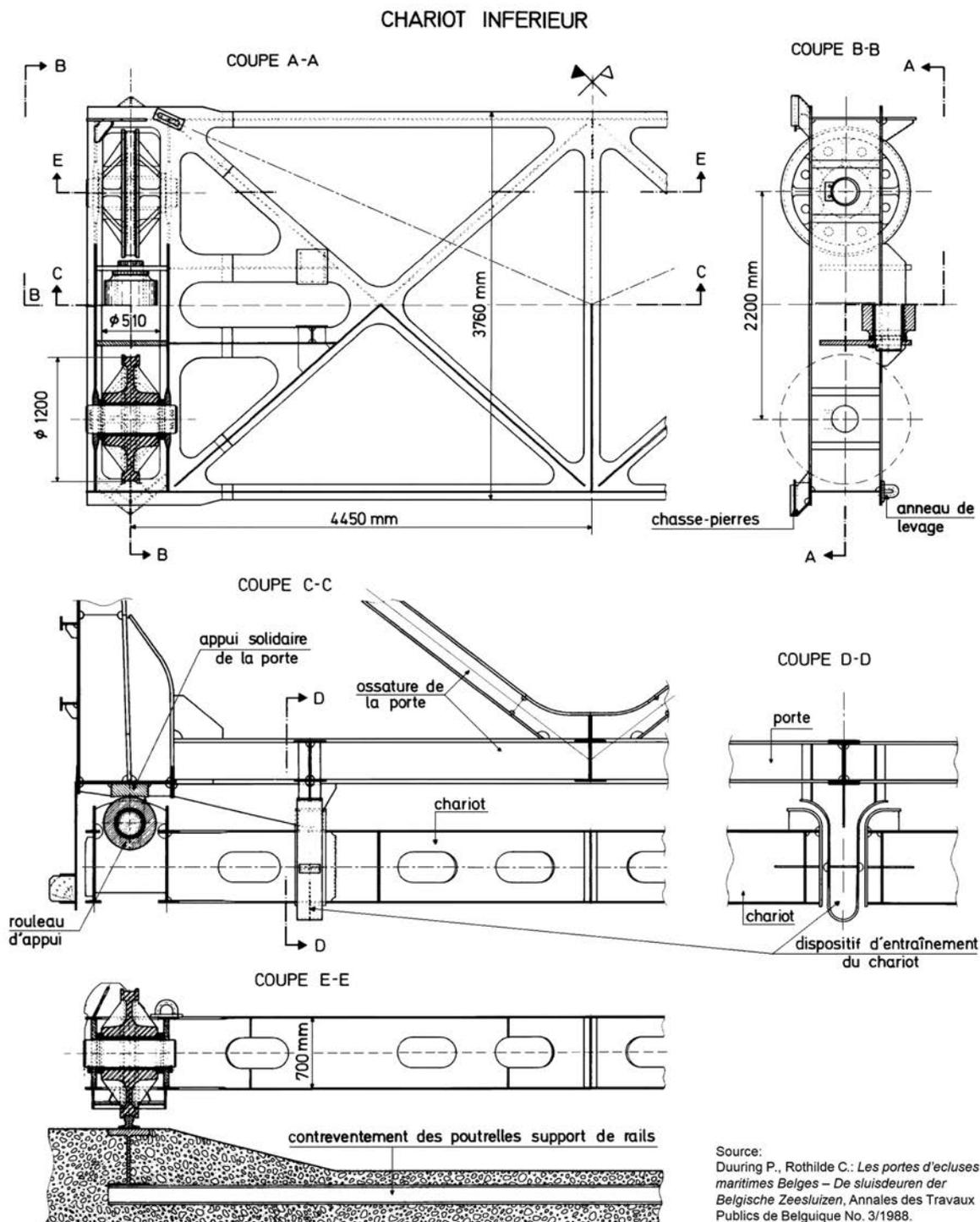
Fig. 12. Lower carriage of the Berendrecht Lock gates [11]
