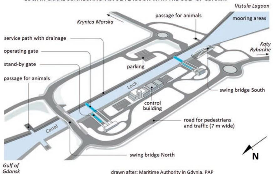
Fig. 3. Lock in Vistula Spit Canal, under construction, general layout
