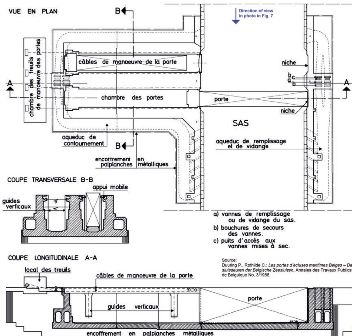
Fig. 6. Typical lock head with rolling gates in Belgium [11]
