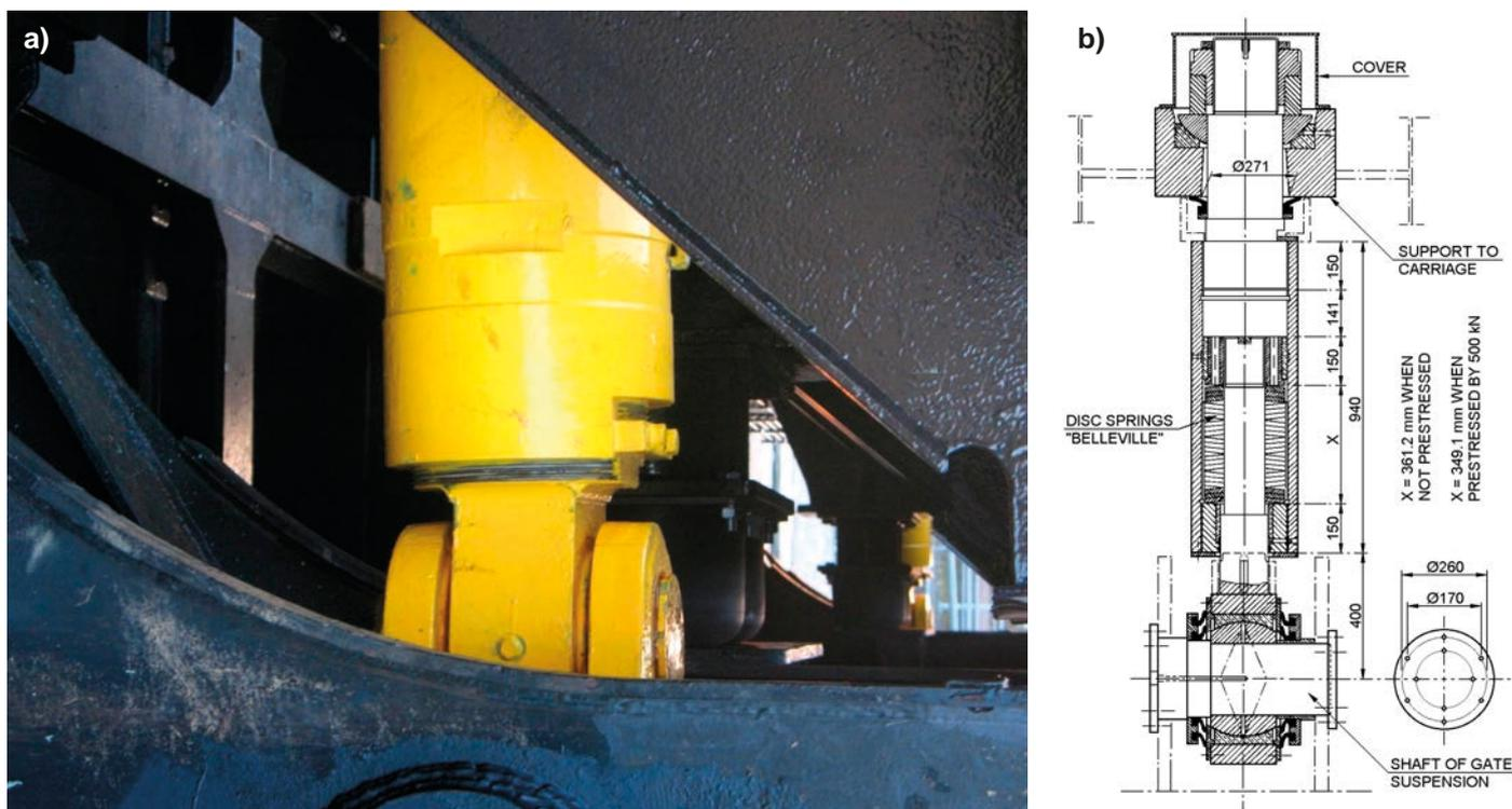
Fig. 13. Suspension of the Zandvliet and Berendrecht Lock gates to upper carriage: a) spring-disc hangers on gate, photo R. Daniel, b) typical Belleville hanger [1, 11]
