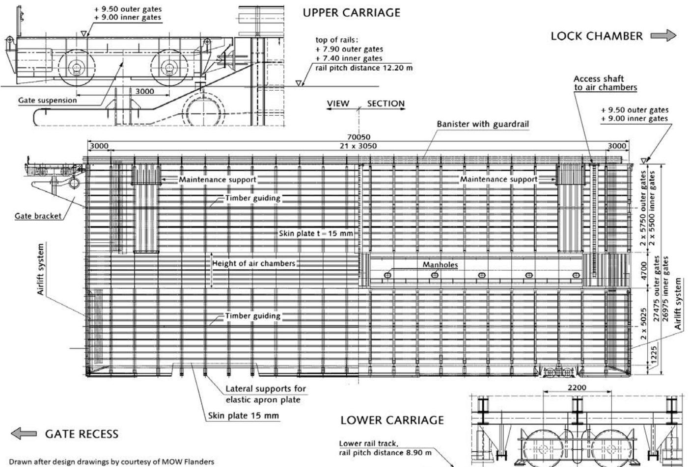
Fig. 10. Rolling gate and its carriages in Kieldrecht Lock, Antwerp [1]
