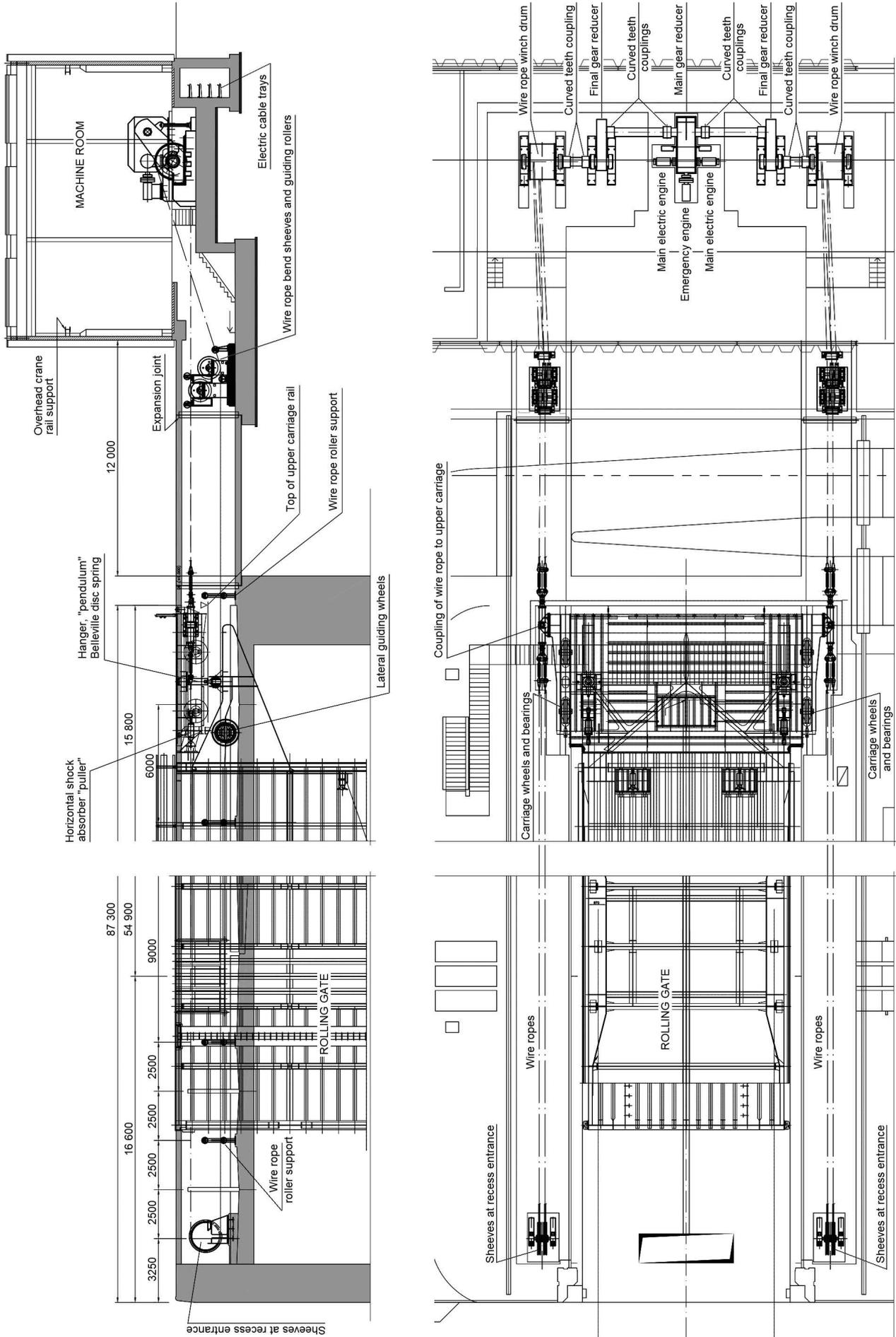
Redrawn from: 2e Sluis Waaslandhaven Antwerpen, Deurmechanismen - Samenplan, drawing EMT 3972-1, by courtesy of Port of Antwerp, 20-08-2010.
