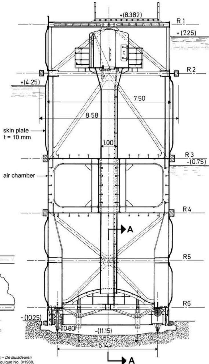
Fig. 11. Rolling gate of the Boudewijn Lock in Antwerp, cross-section [1]
