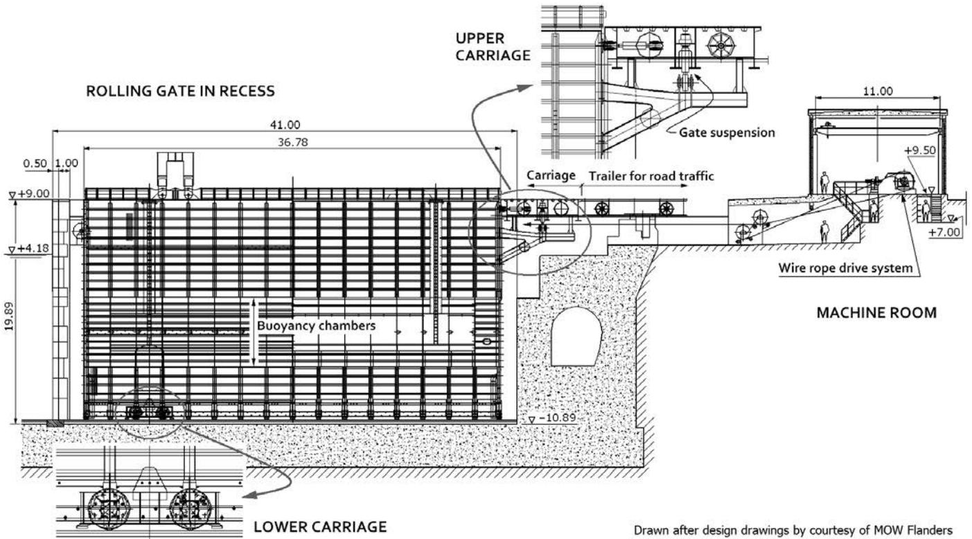
Fig. 9. Rolling gate and its drives in Van Cauwelaert Lock, Antwerp [1]
