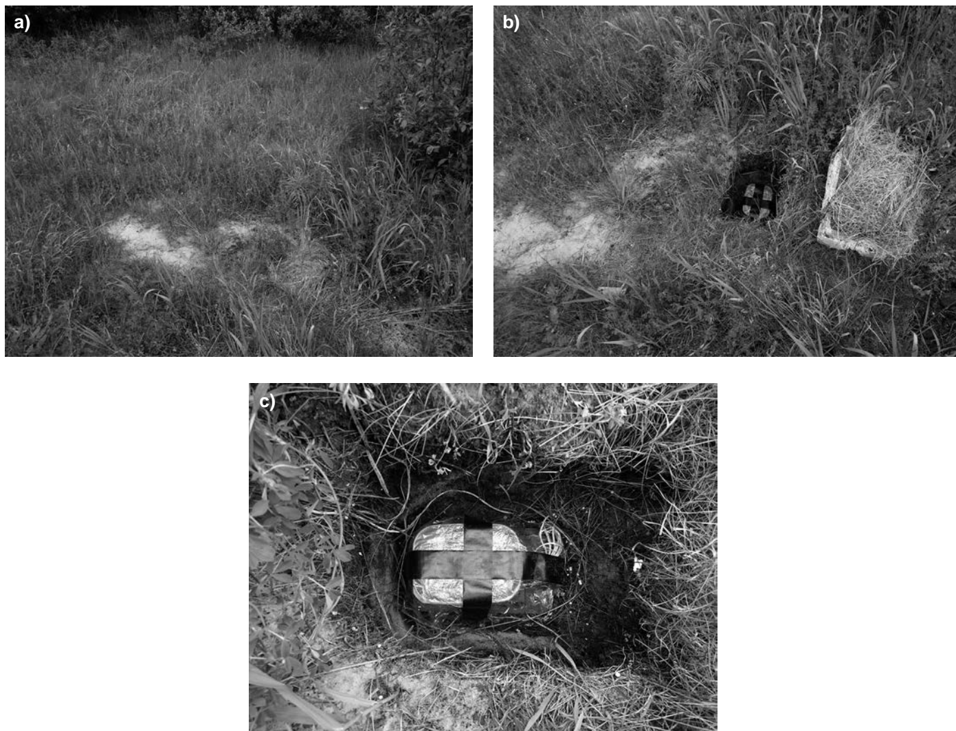
Fig. 5. View of the research field; a) masked research site; b) clipboard with IoT module; c) installed IoT module.
