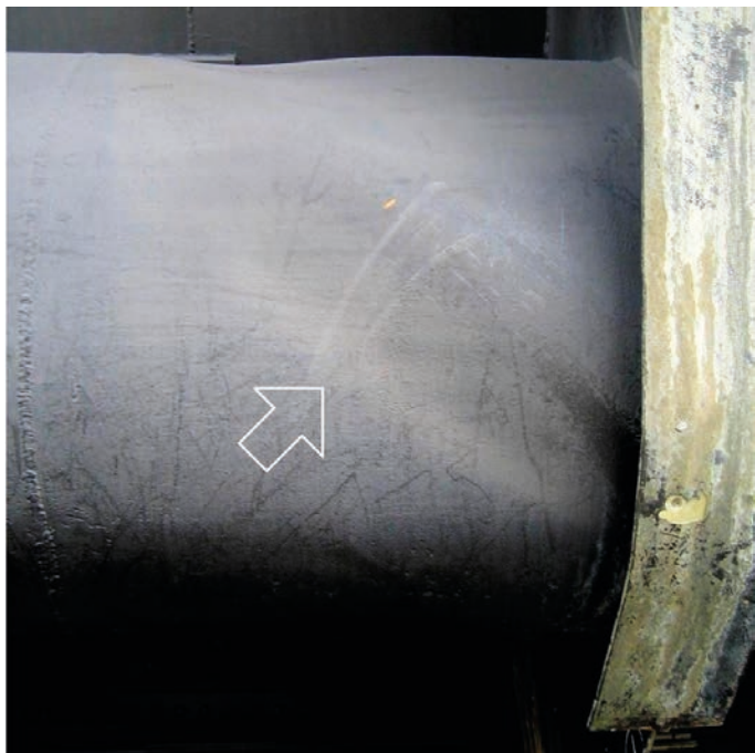
Fig. 14. Lith Weir gate damages, details, photos Rijkswaterstaat a) deformed torque tube of the flap section, b) fractures of flap lever arm castings
