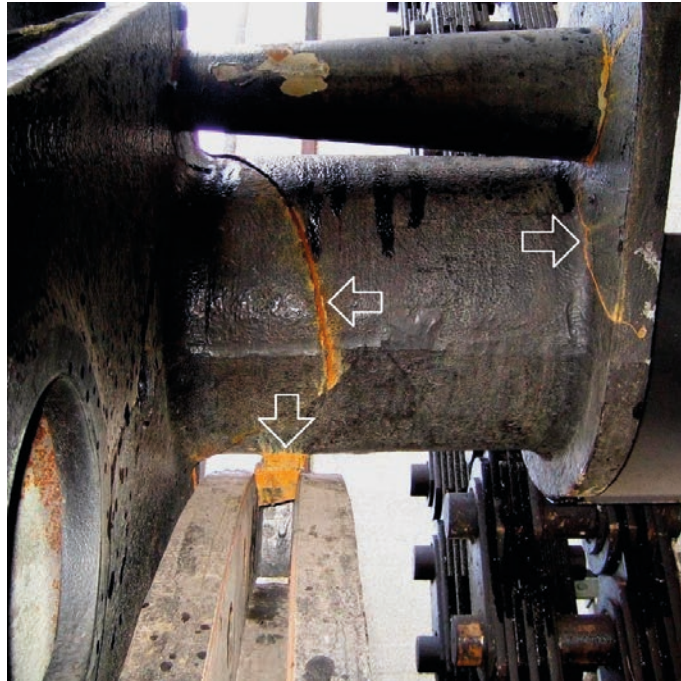
Fig. 14. Lith Weir gate damages, details, photos Rijkswaterstaat a) deformed torque tube of the flap section, b) fractures of flap lever arm castings
